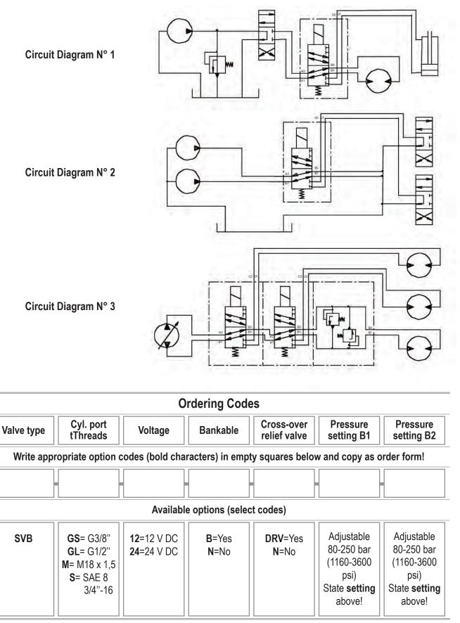
By means of an appropriate assembly kit, the SVB03/SVB04 valves can be banked to obtain e.g. 3 ways from two valves, etc. When marking "B" in the "Bankable" ordering square, an assembly kit is automatically delivered.
