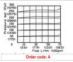
Relief anti-cavitation valve. Works as both port relief and anti-cavitation valve.
