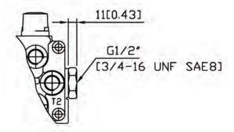
**Tank port reduction adaptor,** can be installed in the T1 port when the thread size is to be reduced from BSP 3/4" to BSP 1/2" or from SAE12 to SAE 8.
