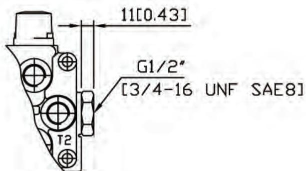
**Tank port reduction adaptor**, can be installed in the T1 port when the thread size is to be reduced from BSP 3/4" to BSP 1/2" or from SAE12 to SAE 8.
