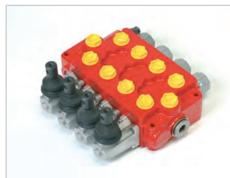
**The CV 400 Unibody** is a modular monoblock valve which is available in 1 to 4 sections, with the option of additional spool functions by using a carry-over fitting (Power Beyond). The valve is designed for a maximum working pressure of 320 bar (4600 psi) with a flow from 15 to 80 l/min (4-21 USgpm).
