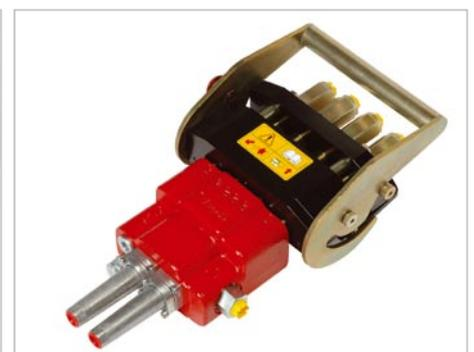
**The CV 152** is a two spool mono block valve specially designed for small and mid size loader applications. It is designed for both open center and load sensing hydraulic systems. The open center version can also be converted to a constant pressure system.
