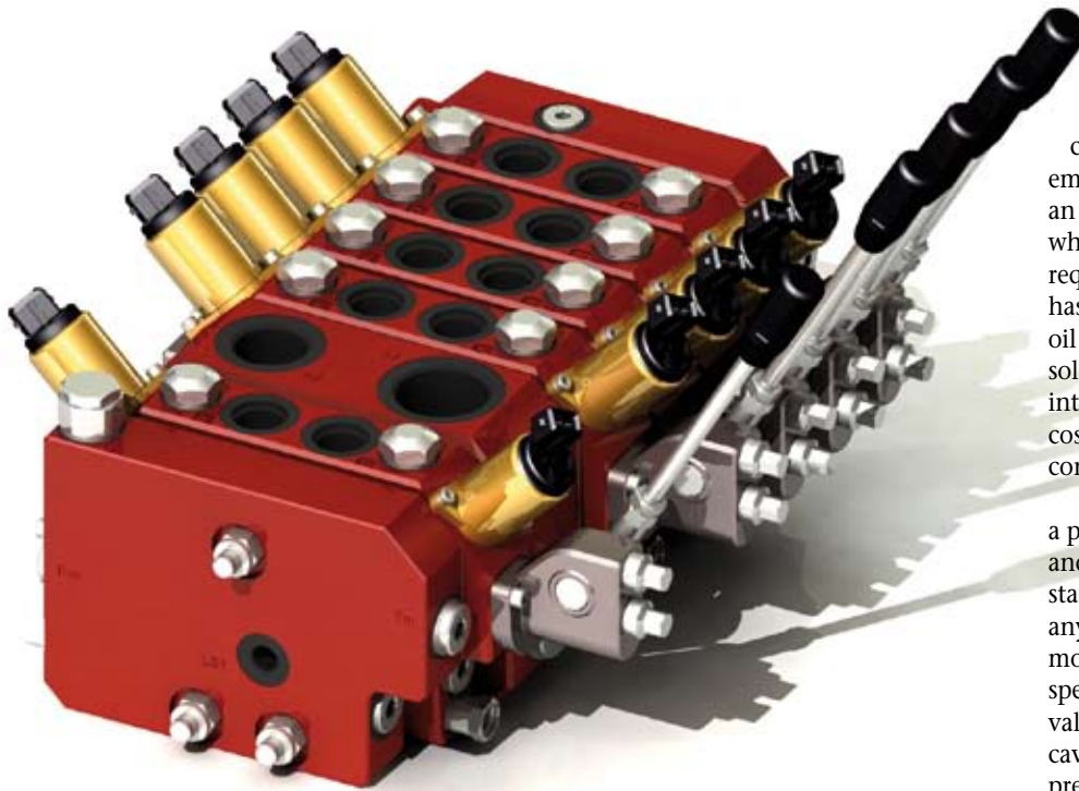
ABOVE: CV2000LS post pressure-compensated control valve, equipped with mid-inlet module for high inlet flows and electrohydraulic actuation
